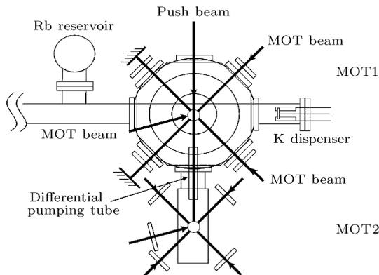
**Fig. 1.** Experimental apparatus: atoms of both species are cooled and trapped in MOT1 and then transferred in MOT2, where they are magnetically trapped. In the magnetic trap, the potassium sample is cooled to quantum degeneracy by means of efficient elastic collisions with the evaporatively cooled  $^{87}\text{Rb}$ .
