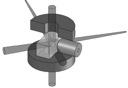
**Fig. 2.** Dual-species MOT2 formed at the intersection of six laser beams. After molasses and optical pumping, the Ioffe coil (purple) converts the spherical quadrupole trap into an Ioffe configuration trap with its trap centre close to the Ioffe coil.
